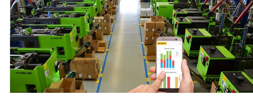
processes (assembly, sorting, testing, etc.) and makes a real-time correspondence between the number of items produced, the time required to produce them and the remaining shift time available, to enable the operator to justify any unproductive periods before the end of his shift.
